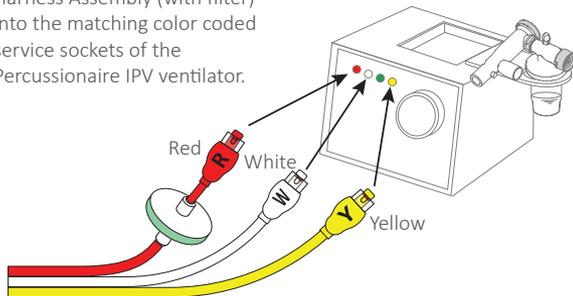
**!** Match color codes of Ventilator End of the Harness Assembly to the IPV ventilator.
