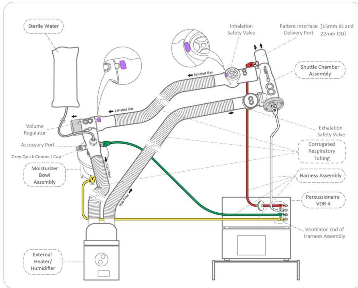
**Full set up of CLV-213 with the VDR-4, the external Heater Humidifier and the sterile water source**
